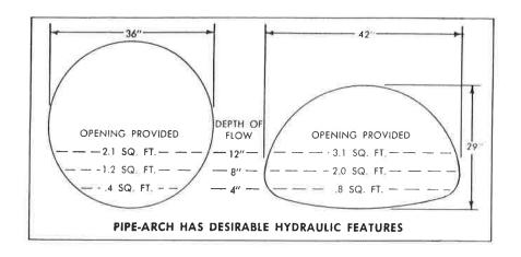
The above example illustrates a 36" round pipe reformed into a 29"  $\times$  42" pipe-arch. At low flows it offers a wider channel to carry more water.
