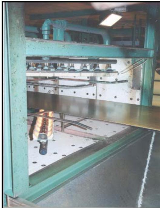
The sheet then goes through a 100-foot-long gas-fired oven to heat the sheet to 400°F.
