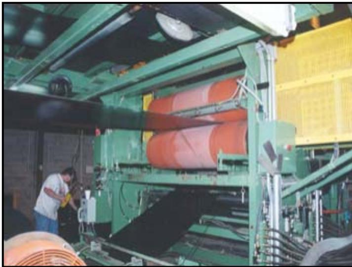
The nip roll pressure is held at 100 psi. The combination of the heat of the steel sheet and the pressure from the nip rolls produces an excellent chemical and mechanical bond of the TRENCHCOAT Film to the galvanized steel.
