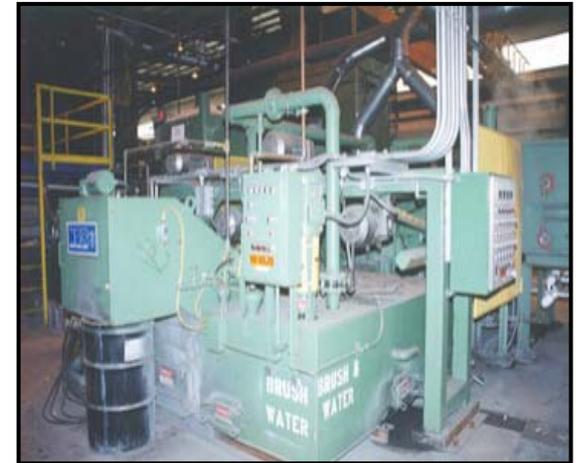
The sheet moves through a double freshwater rinse tank that is continuously filtered. The coil then passes through squeegee rolls to remove the excess water.
